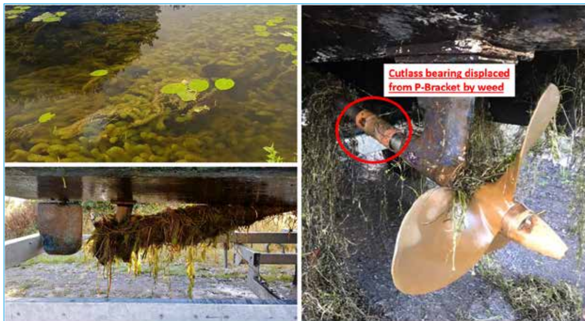
Figure 8 - Excessive weed can have a destructive effect on the engine or stern gear of vessels
